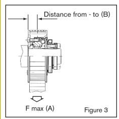
Center the drive element (i.e. timing belt pulley or gear) onto the connecting flange of the MTL and fasten with screws. If the center of the radial load falls over the middle of the MTL an additional support bearing is not required. (Figure 3). Please observe the maximum allowable radial load for each MTL sized as indicated in Table 3. Excess radial load will affect the performance of the MTL.
