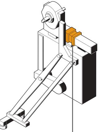
Function: The servomotor brake holds each joint securely to prevent any arm movement during power-off situations.
