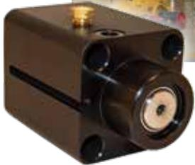
engaged state, several compression springs push on a piston, causing a clamping collar to lock onto the rod. If air pressure is lost, the unit will default to the lock-engaged state. When air pressure is applied, the piston will push back against the springs, releasing the clamping collar. A large clamping area prevents wear on the piston rod. They meet IP67 standards and can be equipped with sensors to detect engagement and disengagement.
