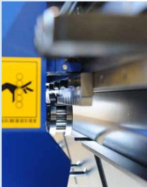
Because of the Nexen Roller Pinion System's low friction operation, it has an unlimited run length. Lack of friction means heat is not generated, which usually leads to component wear. This provides a long equipment life span and low maintenance needs. In most cases, it only needs lubrication every two million pinion revolutions, or approximately six months. In certain applications, it can even operate without lubrication, leading to minimal sacrifice in life.
